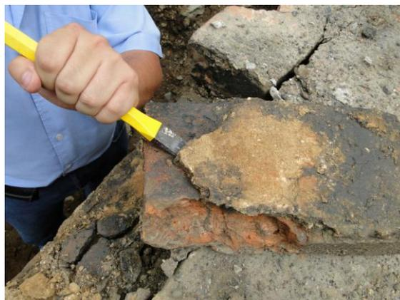
Fig. 3. *Sample extraction of the mortar paste at Puente Ortiz.*
